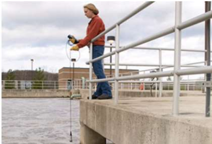
Fig 26 spot sampling an aeration basin
