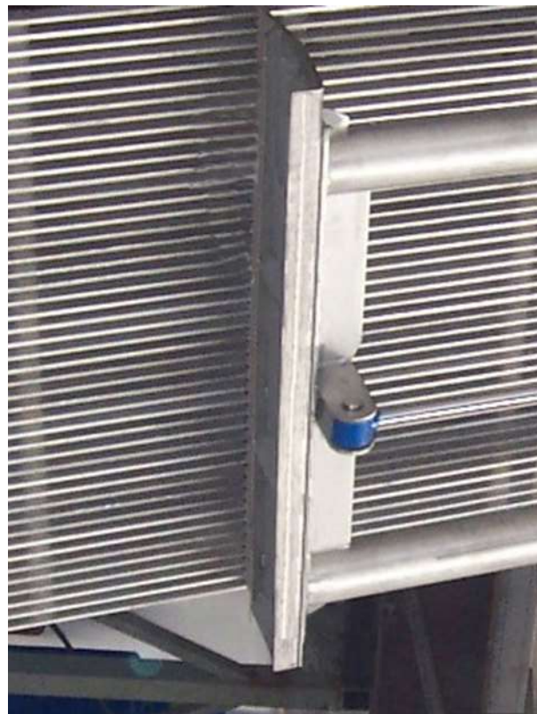
Fig15 A coarse screen
